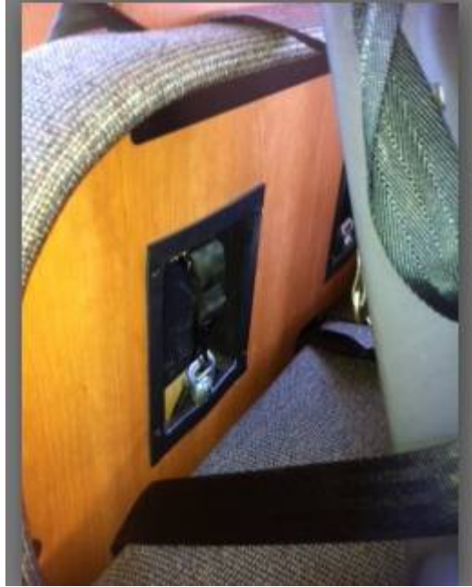
4) Top tether attached to lower anchor
