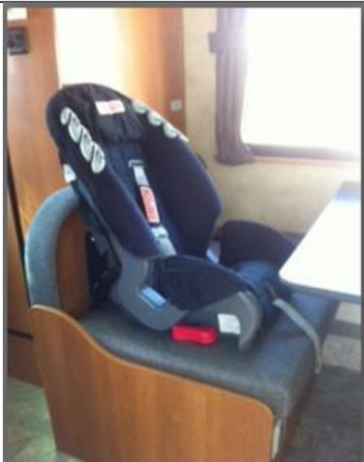
3) Child seat being installed. Tether and lap belt attached (but not cinched)
