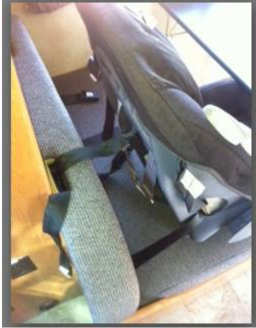
3) Child seat being installed. Tether and lap belt attached (but not cinched)
